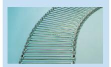
The galvanized conveyor chain consists of two tempered external chains with rods welded in between. The horizontal rods are placed at an even level to ensure that eggs are gently placed on the conveyor, can easily make their way through transfer areas and are not crushed on the inside of bends. Please see the information sheet "Conveyor Chains" for details concerning the applicable conveyor chain angles.
